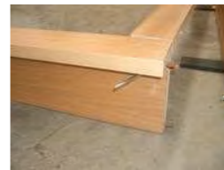
6. Attach head rail to side rails and tighten cam under top of side rail Then attach head panel to side rail and small head rail Tighten cam on inside of side rail then using 3 small bolts attach head panel to head rail Attach adjustable upholstered headboard to back panel with 4 long bolts
