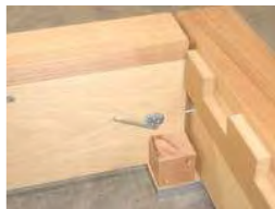
5. Connect foot end to side rails and tighten cams – 1 inside foot end & one underneath top of side rail
