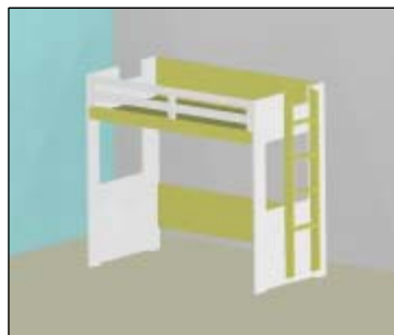
Step 5 Insert mattress base with 4 x 35mm screws
