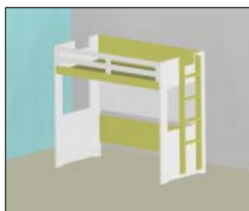
Step 6b Connect desk backing with 4 x silver bolts. Note- the bolts connecting the rails should be loosened, BUT still threaded.
