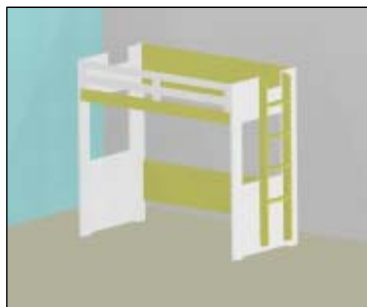
Step 4 Connect ladder with 8 x 40mm silver bolts
